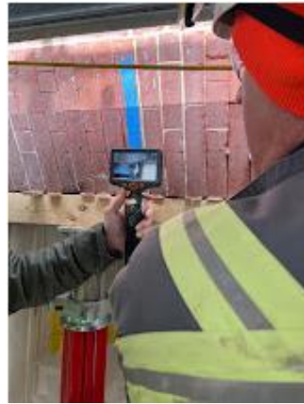
Investigation of concealed spaces using pin-hole camera
